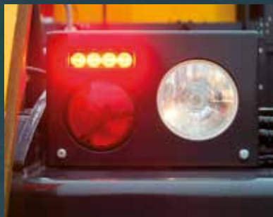
Rear flashing lights supplement the audible warning signals for the safety of those inside and outside the cab.
